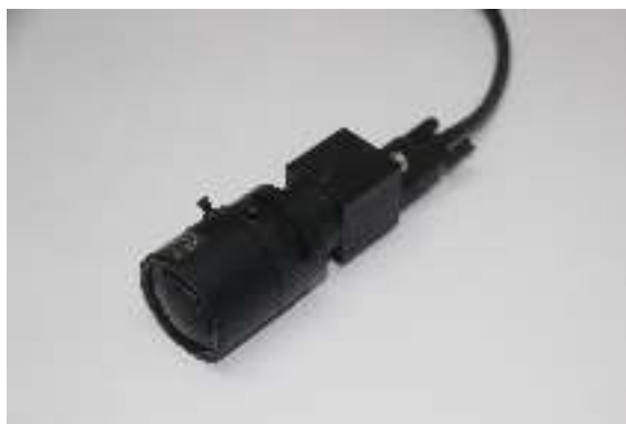
Figure 2.1: Point Grey FL3-U3-13Y3M-C camera.
