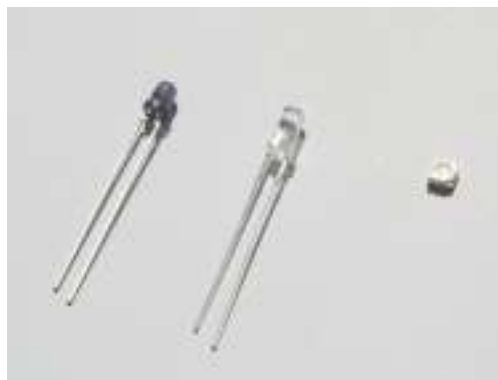
Figure 3.1: Infrared LEDs from left to right: Osram SFH 409, Harvatek HE3-1100AC and OptoSupply OSI3NAS1C1A (SMD).
