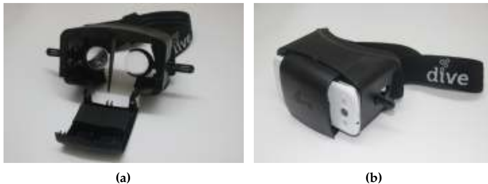
Figure 5.1: The head-mounted device Durovis Dive without display (a) and with an inserted smartphone (b).
